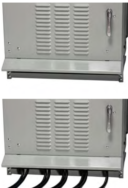
Bottom Door and Cables (Type 3R) The Hinged Cable Entry Trap Door Allows Cable Access to Both the Receptacles and Lugs, While Maintaining Type 3R Enclosure Integrity
